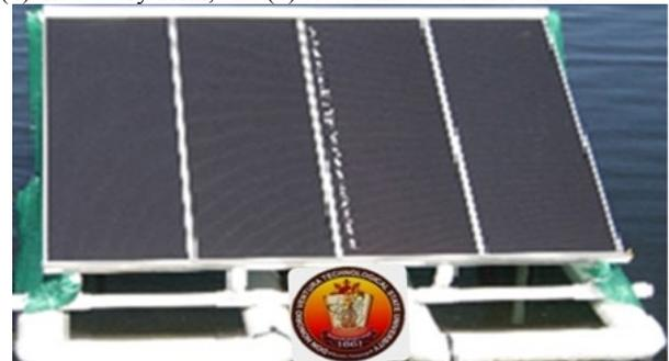
Fig.1: The completed modified solar powered pond aerator assembly
