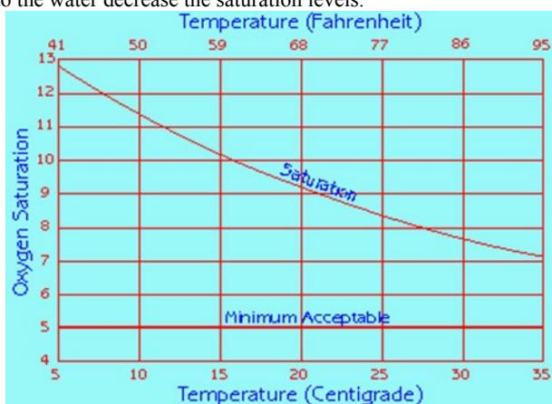
Fig. 5: Oxygen Saturation vs. Temperature
