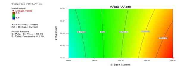
Fig. 6e: Weld width-(Pulse on time-60% & pulse frequency-5Hz)
