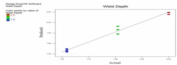
Fig.4b: Experimental value vs. predicted value for weld depth
