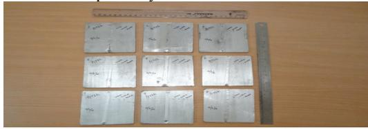
Fig. 2: Welded samples of PCTIG welding
