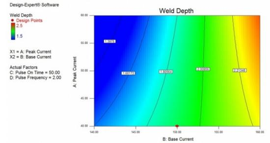
Fig. 5a: Weld depth-(Pulse on time-50% & pulse frequency-2Hz)
