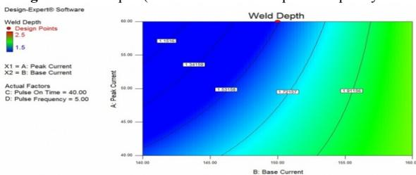
Fig. 5d: Weld depth-(Pulse on time-40% & pulse frequency-5Hz)
