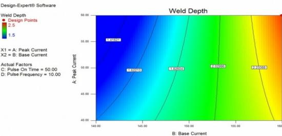
Fig. 5c: Weld depth-(Pulse on time-50% & pulse frequency-10Hz)
