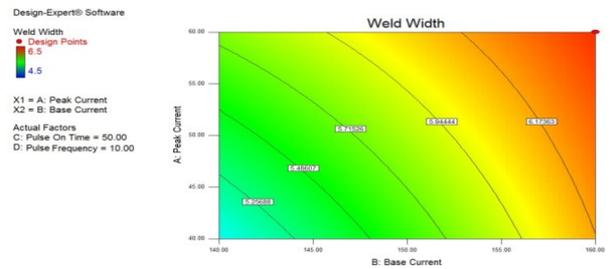
Fig. 6c: Weld width-(Pulse on time-50% & pulse frequency-10Hz)
