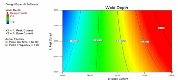
Fig. 5e: Weld depth-(Pulse on time-60 & pulse frequency-5Hz)
