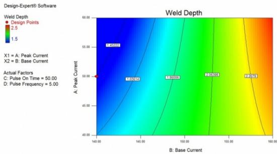
Fig. 5b: Weld depth-(Pulse on time-50% & pulse frequency-5Hz)
