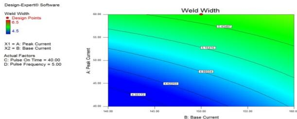
Fig. 6d: Weld width-(Pulse on time-40% & pulse frequency-5Hz)
