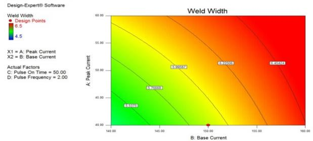
Fig. 6a: Weld width-(Pulse on time-50% & pulse frequency-2Hz)
