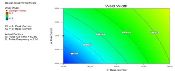
Fig. 6b: Weld width-(Pulse on time-50% & pulse frequency-5Hz)
