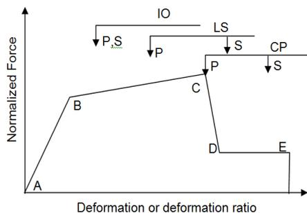
Fig. 2: Idealized force-deformation curve
