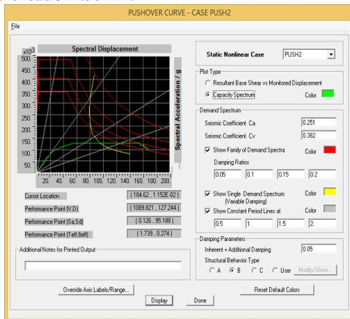
Fig.6: Capacity spectrum curve for EQ-X dir
