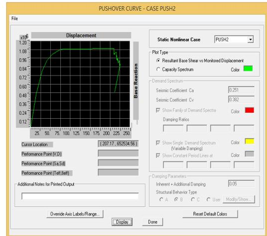
Fig.7: Resultant Base Shear vs Displacement
