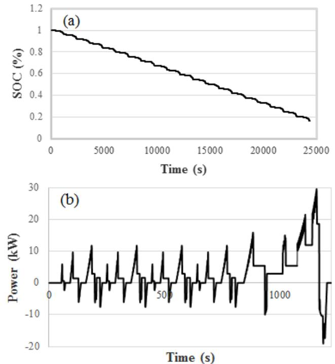
Fig. 2: (a) New European Driving Cycle (NEDC), (b) Power to complete a driving cycle.
