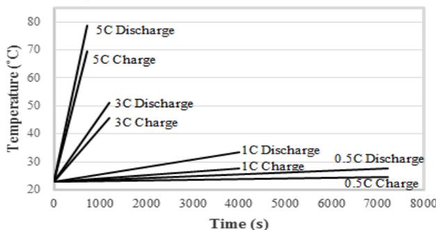
Fig. 1: Battery temperature during different charge and discharge rates.
