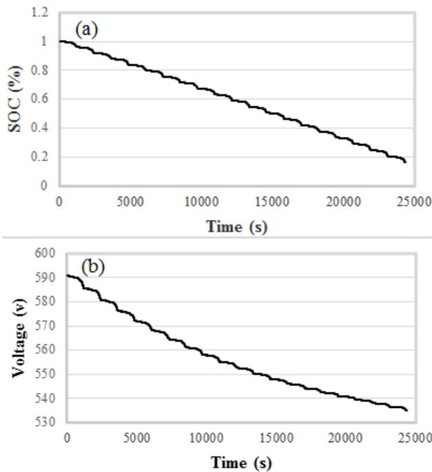
Fig. 3: (a) Battery SOC, (b) Battery output voltage to complete 20 NEDC cycles.
