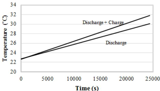
Fig. 4: Battery temperature with consideration heat generation during charge and discharge.
