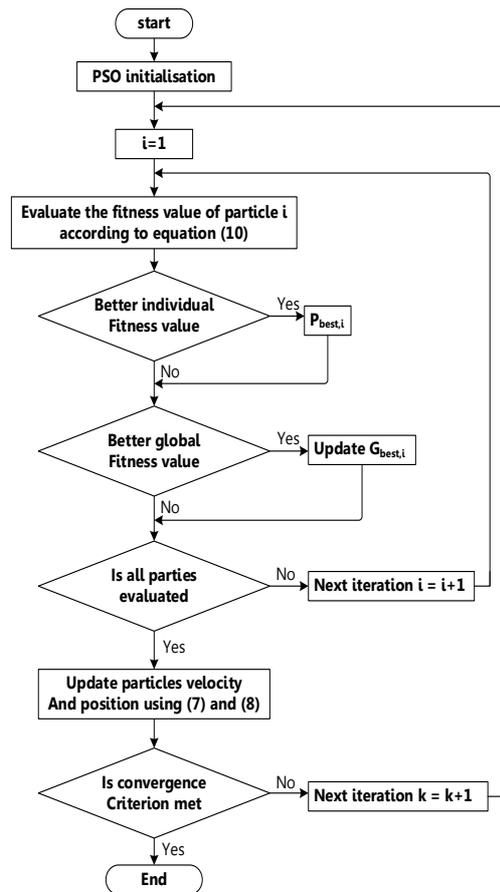
Fig.3. Flowchart of the PSO algorithm for variable-angle PS-PWM
