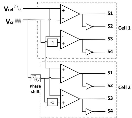
Fig.2. PS-PWM generator diagram of two cells CHB-MLI
