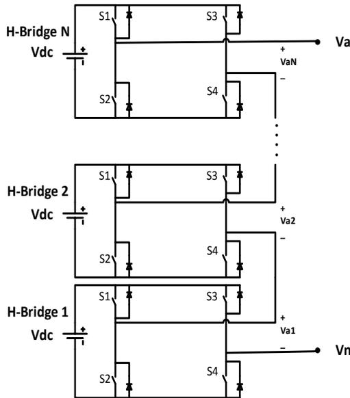
Fig.1. Structure of a single-phase n-level CHB-MLI
