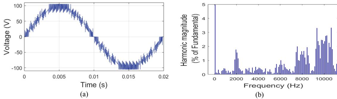
**Fig.7.** Result of the adapted PS-PWM based on PSO algorithm with unequal dc-links voltage for eleven-level inverter: (a) Output voltage waveform; (b) harmonic spectrum.
