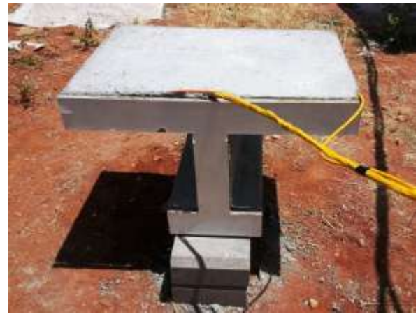
Fig. 2: The experimental girder segment (a) The formwork and the installation of the thermocouples, (b) the final view
