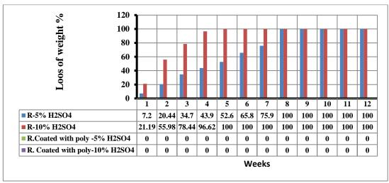
Figure 5: Explain the loss of weight for reference specimens coated with polyurethane immersed in diluted sulfuric acid with weeks.
