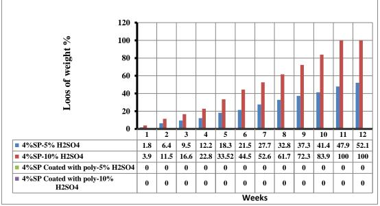
Figure 6: Explain the loss of weight for 4%SP specimens coated with polyurethane immersed in diluted sulfuric acid with weeks.
