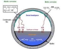
Figure 1: Mechanism of Biogenic Sulphuric Acid Corrosion
