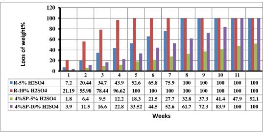
Figure 4: Explain the loss of weight for reference and 4%SP mix immersed in diluted sulfuric acid with weeks.
