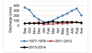
Fig. 3: Inflow from the Tigris and the Euphrates rivers to Shatt al-Arab river in three different water years. The pre-regulation flow is represented by the year 1977-1978.
