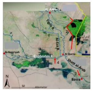
**Fig. 8**: Proposed engineering works in the lower Euphrates and Tigris as part of Shatt al-Arab remediation plan. The numbers designate the engineering modification as in section (6)
