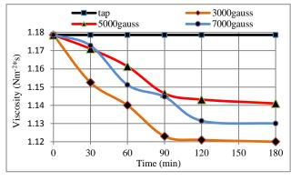
Fig. 6: Magnetic field effect on the viscosity of water
