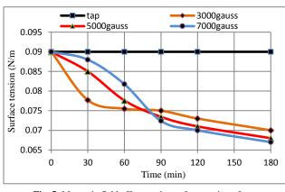
Fig. 5: Magnetic field effect on the surface tension of water
