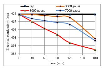
Fig. 7: Magnetic field effect on E.C. of water
