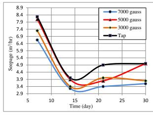
Fig. 11: Magnetized water effect on the seepage of concrete
