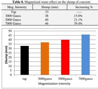
Fig. 9: Magnetized water effect on the slump of concrete
