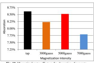
Fig. 10: Magnetized water effect on the absorption of concrete
