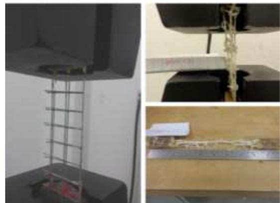
**Fig. 2:** Test instrumentation of (1) steel specimen (left), (2) #15 FN (right) [28].
