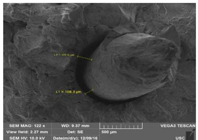
Fig. 13: WWSM yielding before the wire failure (Section A) [28].
