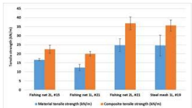
Fig. 8: Material and composite tensile strength of FN and WWSM [28].
