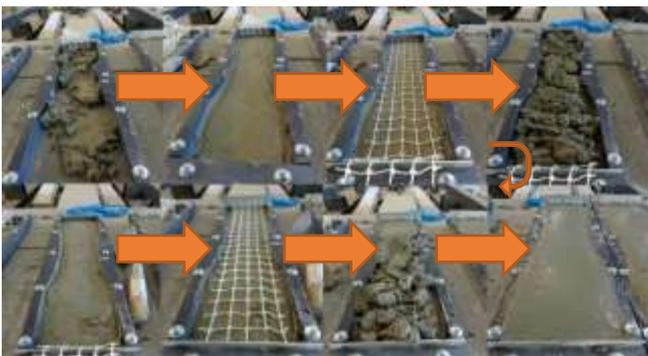
Fig. 5: Casting procedure of the dog-bone specimens [28].
