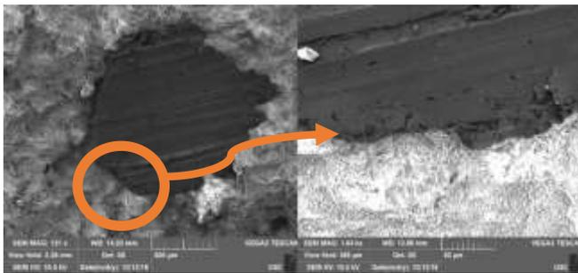
Fig. 15: A steel wire at the new cut section (Section B) [28].
