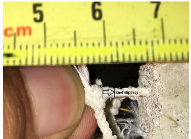
Fig. 12: FN slippage from the knot (Section A) [28].
