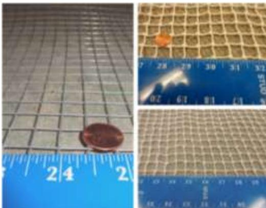
**Fig. 1:** Welded wire steel (left) and #21 FN mesh (right) spacing [28].
