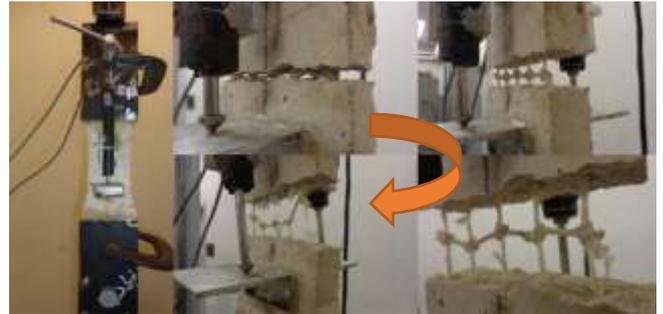
Fig. 7: A dog-bone composite specimen (#21 FN, 1 layer) under uniaxial tensile test [28].
