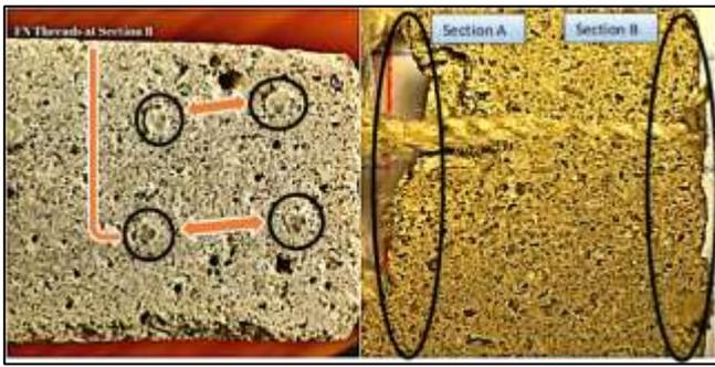
Fig. 14: FN threads impregnation by the mortar at section B [28].
