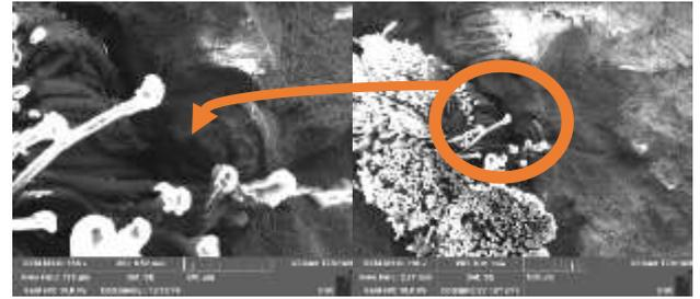
Fig. 11: FN thread impregnation by the mortar, the photo captured by using the SEM microscope [28].
