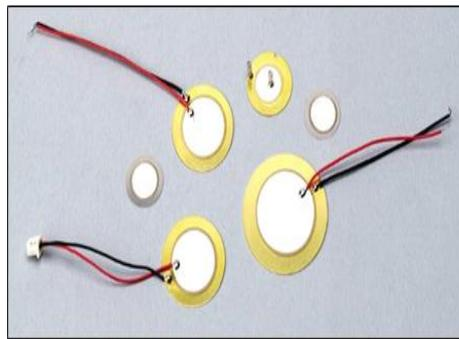
Figure 2: Piezoelectric Disk
