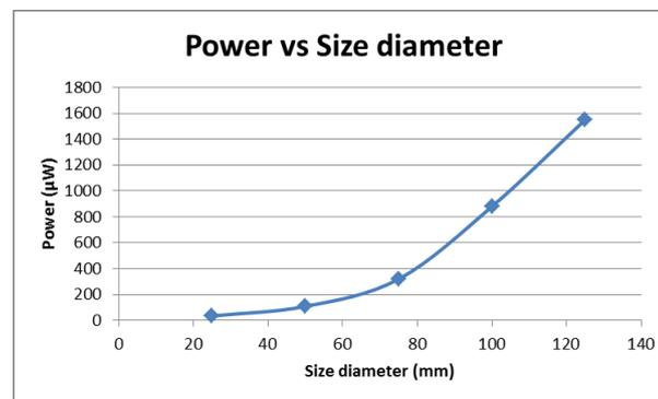
**Figure 12:** Power produced by prototype generator of different diameters
