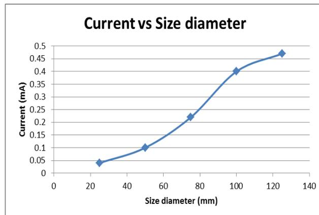
**Figure 10:** Output current produced by different diameter of piezoelectric transducer
