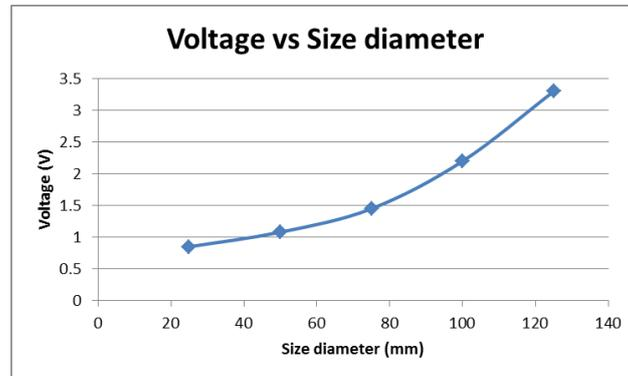
**Figure 9:** Output voltage produced by different diameter of piezoelectric transducer
