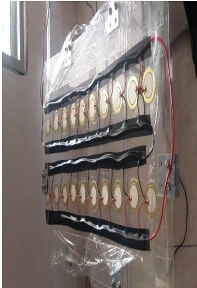
**Figure 6:** Hardware development for Hardware piezoelectric transducer roof
