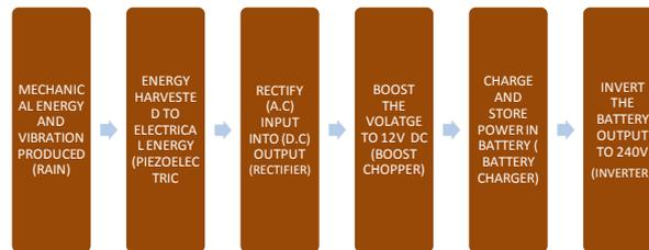
Figure 1: Block Diagram of raindrop power generator module
