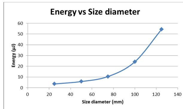
**Figure 11:** Energy produced by prototype generator of different diameters
