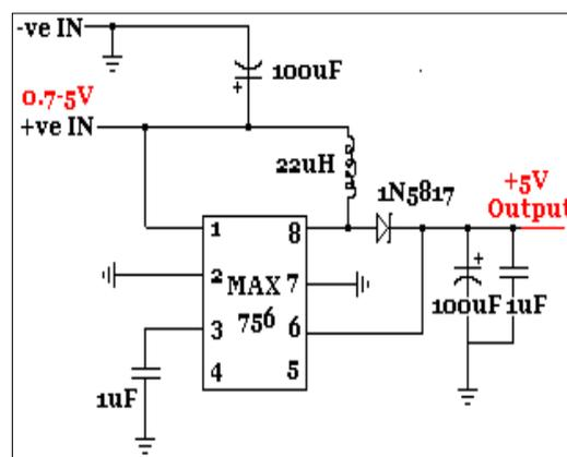
Figure 3: DC Boost Converter
