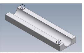
Fig. 4: Isometric view of the lower mold half with dowel pins
