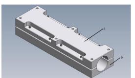
Fig. 3: Isometric view of the molds which were divided into two parts: (a) upper mold half and (b) lower mold half
