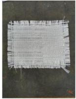
Fig. 1: E-glass fibers in mat form
