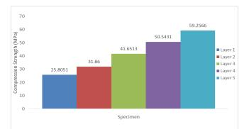
Fig. 11: Comparison of compression strength between the specimens with different layer of E-glass fiber in quasi-static crushing
