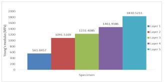
Fig. 10: Comparison of Young's modulus between the specimens with different layer of E-glass fiber in quasi-static crushing
