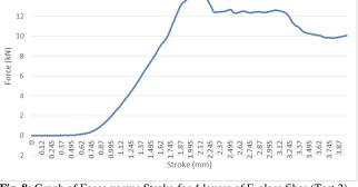
**Fig. 8:** Graph of Force versus Stroke for 4 layers of E-glass fiber (Test 2)
