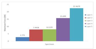
Fig. 9: Comparison of maximum force between the specimens with different layer of E-glass fiber in quasi-static crushing
