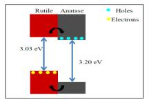
Figure 4 Proposed valence and conduction band alignment mechanism for rutile/anatase interface [87].
