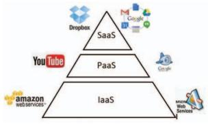
Figure 1: Cloud Computing Layer link to current famous user [2]
