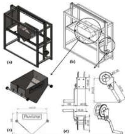
**Fig. 5:** (a) Pictorial view of mechanical pluviator; (b) Schematic view of pluviator; (c) V-shape container and (d) Mechanical chain and rope lever
