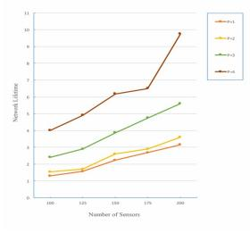
Fig. 1: Network lifetime vs. number of sensors
