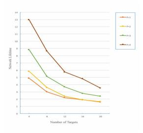
Fig. 2: Network lifetime vs. number of targets
