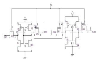
Fig. 4: Fault Model for  $\mathrm{CF}_{\mathrm{st}}$  using Short between QB1 and Q0
