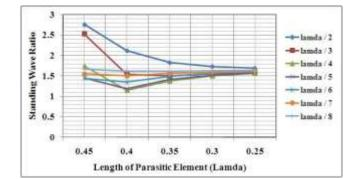
Fig. 3: Variation on SWR on the proposed 408 MHz antenna with two parasitic elements
