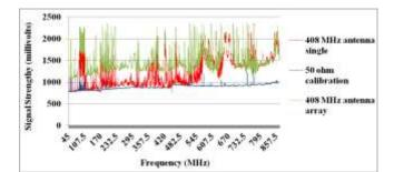
Fig. 8: Comparison on spectral views obtained by utilizing single antenna, array antenna and 50 ohm calibration
