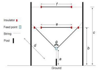
Fig. 1: Geometry of the proposed 408 MHz antenna
