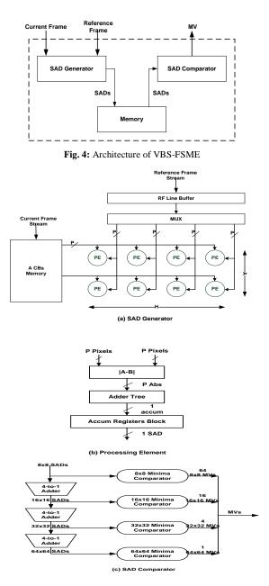
Fig. 5: Functional units of the reconfigurable VBS-FSME architecture
