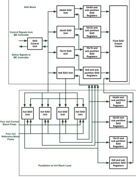
Fig. 3: SAD architecture with parallelism
