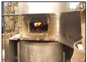
Fig. 2: Incenerating Process in Standing Furnace Incenerator (Incenerator Dapur Tegak)
