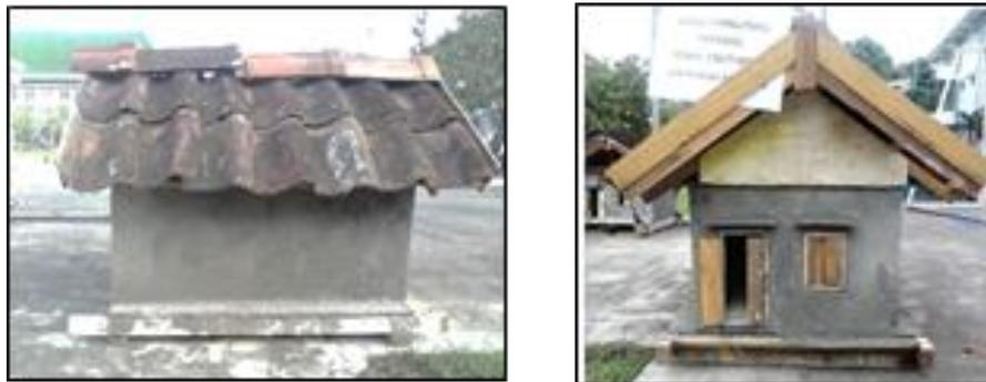
Fig.1: Building mockup with clay tile rooftop
