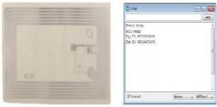
a) Passive RFID Tag b) RFID Tag read through Wearable Fig 6: RFID Module
