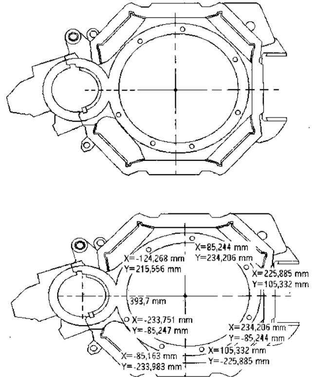
Fig. 2: Axle cap of GE 761 traction motor
