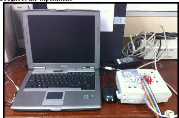
Fig. 5: Neurofax EEG-9200 machine and bipolar jack
