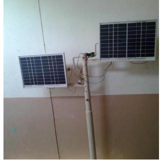
Fig. 10: Time Lapse Based Single Axis MPP Tracking System for Solar Tree front view
