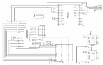
Fig. 8: Main relay schematic diagrams of time lapse solar tracking syste
