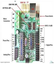
Fig. 2: Atmega 328p Micro Controller
