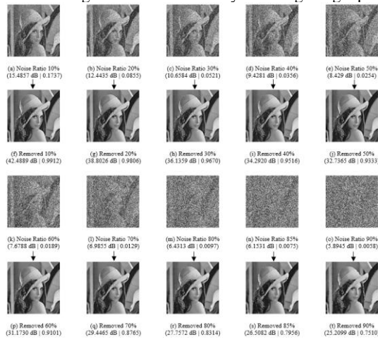
Fig. 10: The Simulation Result of Noisy Images ('a', 'b', 'c', 'd', 'e', 'k', 'l', 'n', 'o') and Respective Filtered Images ('f', 'g', 'h', 'i', 'j', 'p', 'q', 'r', 's', 't').
