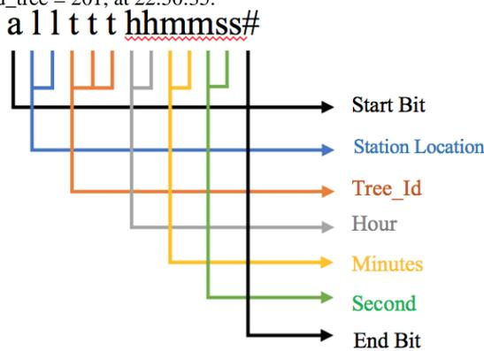
Fig. 5: Log Data Structure for Tracking System
