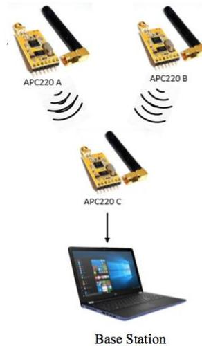
Fig. 2: Wireless Sensor Network Topology Using APC220
