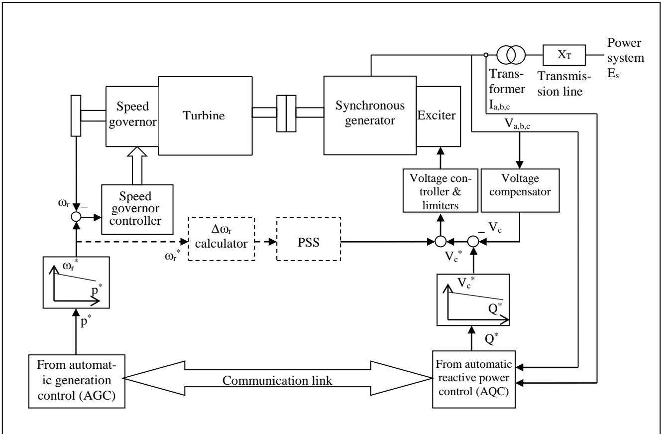
Fig. 1: General synchronous generator control system
