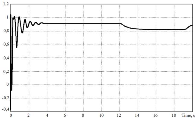
Fig. 12: generator voltage (pu) with Time (s)
