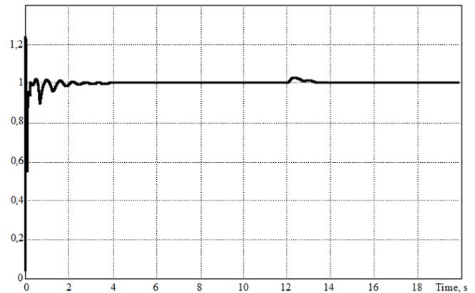
Fig. 4: Generator voltage (pu) with Time (s)
