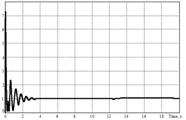
Fig. 9: Generator current (pu) with Time (s)
