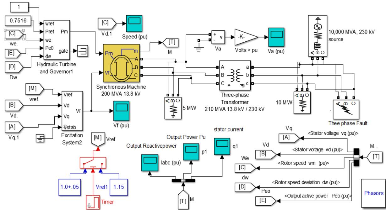
Fig. 3: Hydraulic turbine with Syn. generator
