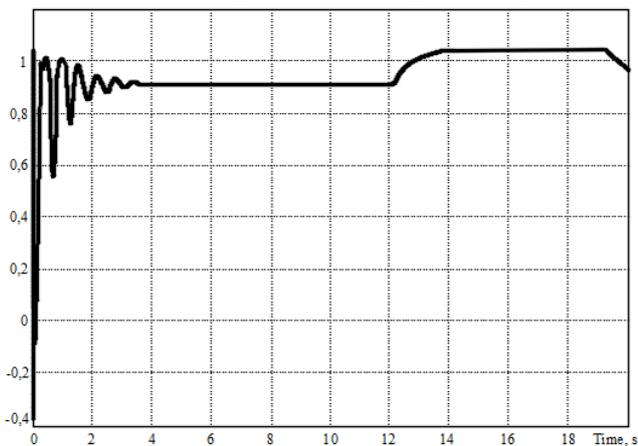
Fig. 8: Generator voltage (pu) with Time (s)
