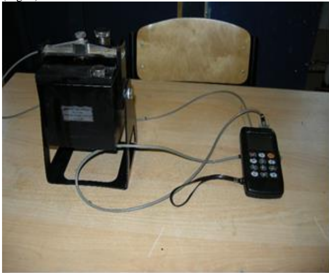
Fig.. 1: Illustration of the dilatometer with the measuring electronic unit
