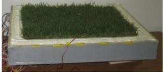
Fig. 1: Model of a "green roof"
