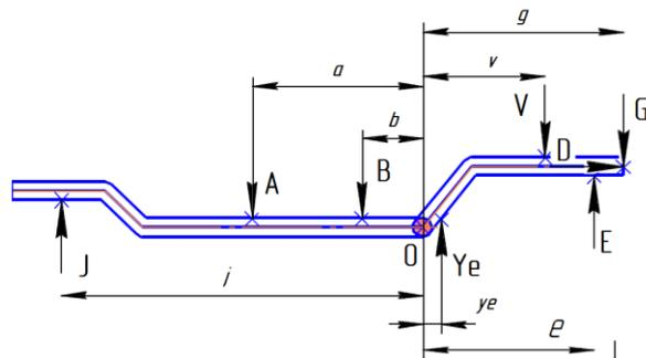
Fig. 7: Scheme of load on the frame
