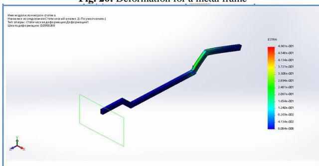
Fig. 21: Deformation for a composite frame
