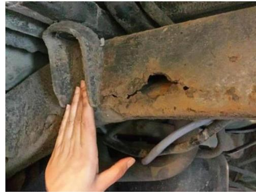
Fig. 3: Damaged frame
