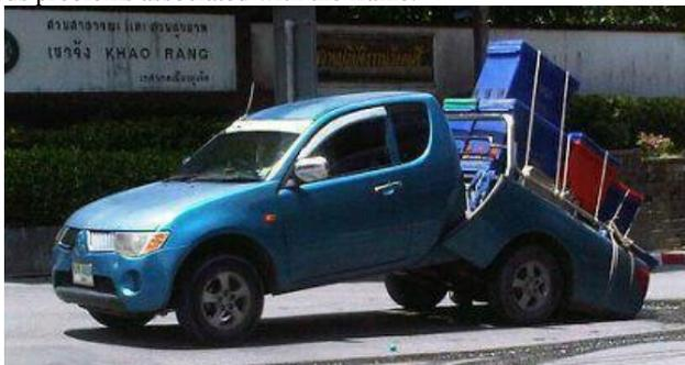
Fig. 2: Illustration of damage to the Mitsubishi L200 IV frame
