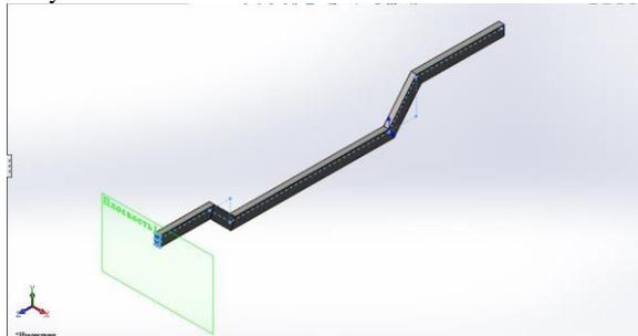
Fig. 12: Model of a spar box frame for static studies
