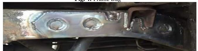
Fig. 5: Refurbished frame
