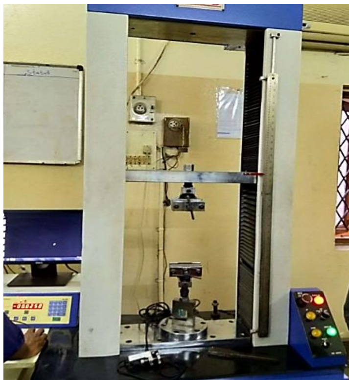
Figure: 7: Mechanical tests conducted on 60T UTM (Tensile Test)
