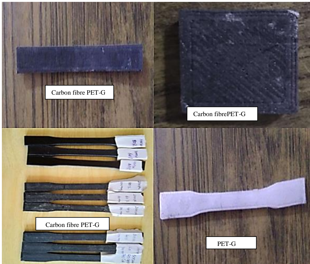
Figure: 5 3D Printed Specimen before testing
