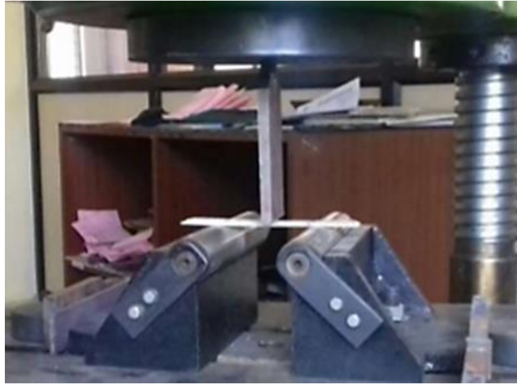
Figure 8: Flexural Testing Machine (60T UTM) Hardness Test
