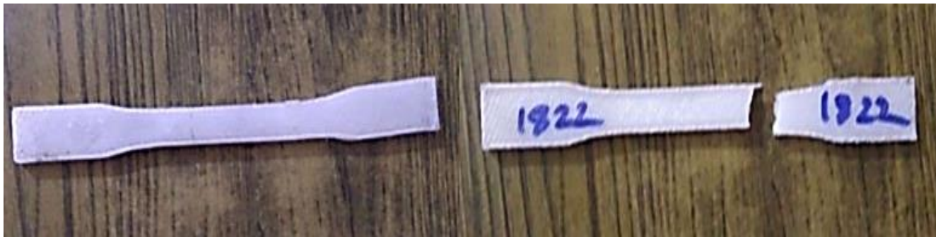
Fig. 11 : Tensile Specimen After Testing ( PET-G)
