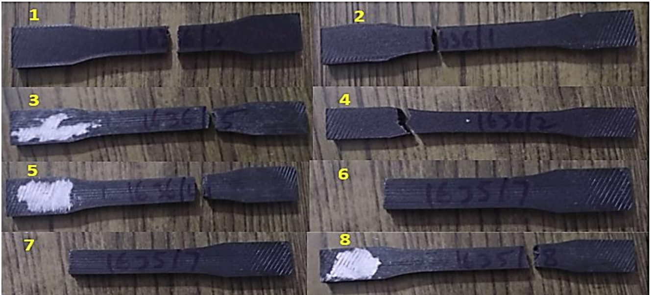
Fig. 10: Tensile Specimens After Testing (Carbon fiber PET-G)
