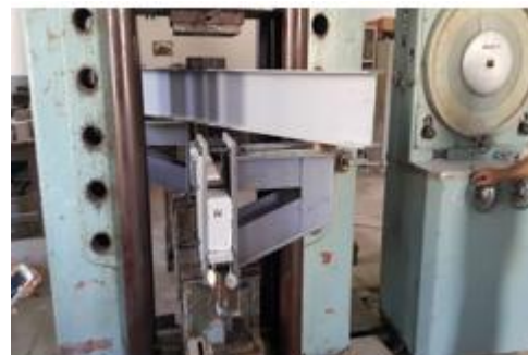
Figure 2: The testing machine and the beam setup
