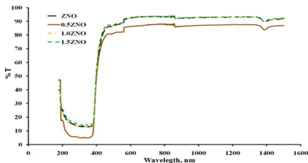
**Fig. 3:** UV-VIS-NIR transmittance against photon wavelength of ZNO, 0.5ZNO, 1.0ZNO, 1.5ZNO samples
