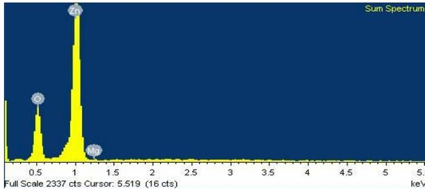
**Fig 2:** The EDX spectrum of ZnO doped with 0.5% of MgO (0.5ZNO) sample.
