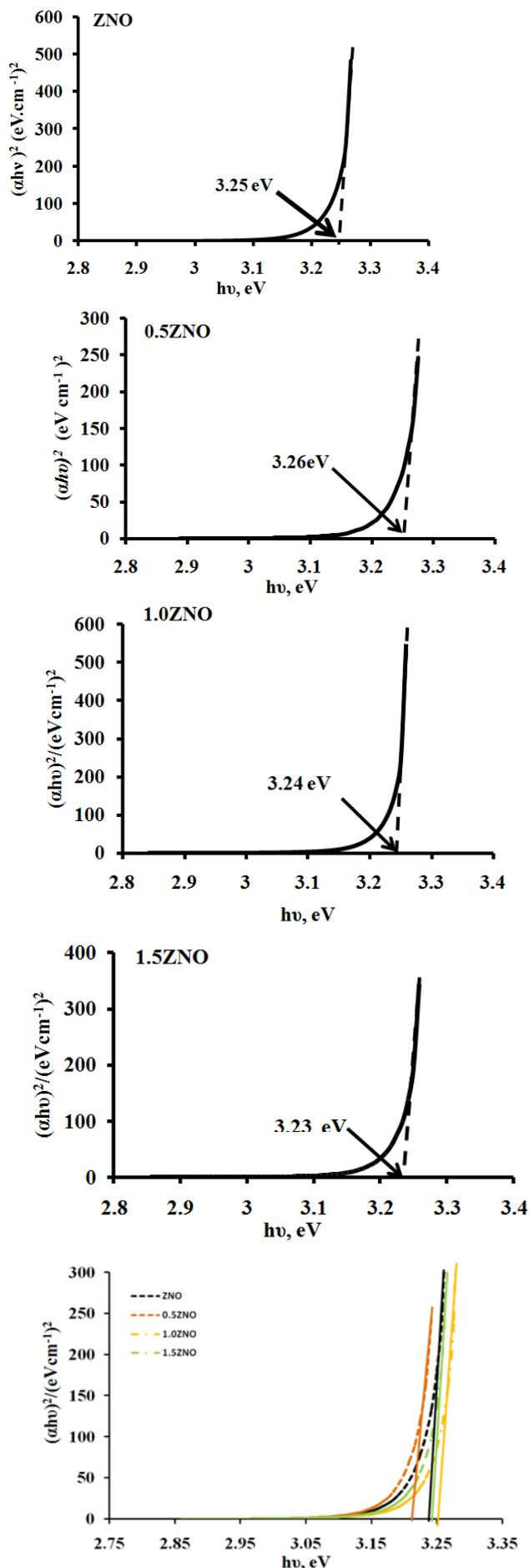
Fig. 5: Tauc plot of ZnO, 0.5ZnO, 1.0ZnO, 1.5ZnO samples and a combination of the four spectrum
