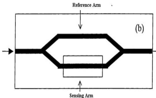
Fig-1: Schematic diagram Of MZI
