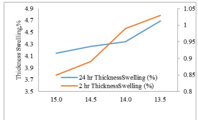
Figure 5: 2 hrs thicknesses swelling of EMDI particleboard at different press factor.
