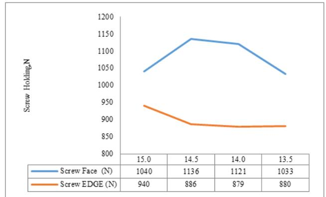
Figure 4: Screw withdrawal Face and Edge of EMDI particleboard at different press factor.
