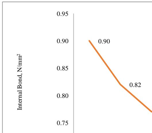
Figure 3: Internal bond of EMDI particleboard at different press factor.
