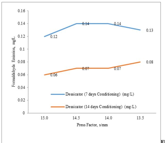
Figure 7: Formaldehyde emission of EMDI particleboard at different press factor.
