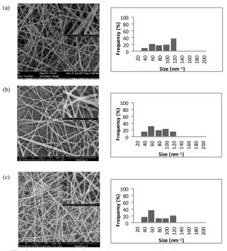
**Fig. 8:** FESEM result of (a) Electrospun PET, (b) Electrospun PET/PR (c) Electrospun PET/PB
