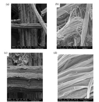
Fig. 6: Surface morphology result of (a) PR (1K x mag), (b) PR (5K x mag) (c) PB (1K x mag) (d) (5K x mag)
