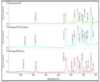
Fig. 7: FTIR result of (a) Electrospun PET, (b) Electrospun PET/PR (c) Electrospun PET/PB
