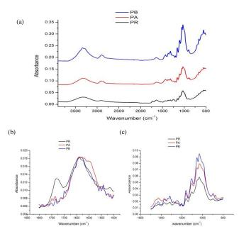
Fig. 3: (a) FTIR spectra of PR, PA and PB (b) zoom in at 1500-1800 cm<sup>-1</sup> (c) zoom in at 800-1500 cm<sup>-1</sup>
