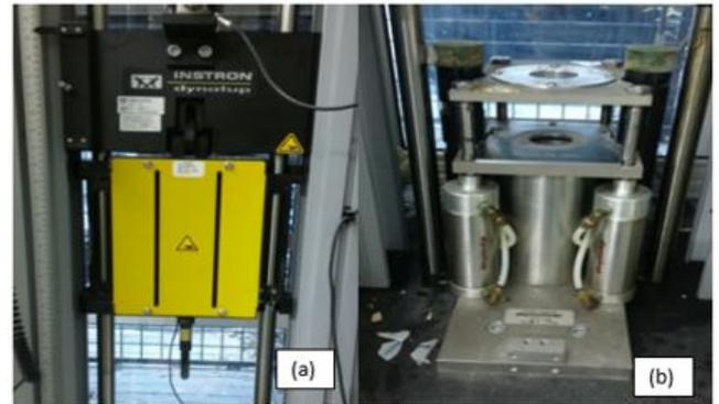
Fig. 5: INSTRON Dynatup 9250 HV (a) and round metal block (b)
