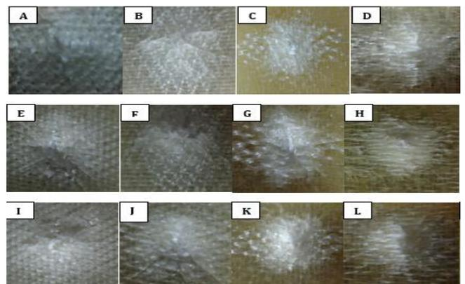
Fig 15: Back Surface Damage on Composites; (A) hemispherical 1A, (B) hemispherical 3AL, (C) hemispherical 4L, (D) hemispherical 9A, (E) conical 1A, (F) conical 3AL, (G) conical 4L, (H) conical 9A, (I) ogival 1A, (J) ogival 3AL, (K) ogival 4L, (L) ogival 9A
