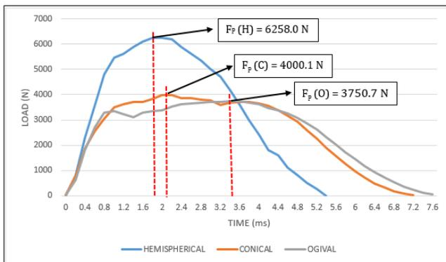
Fig. 9: Peak force over time for all impactor shapes impacted on 4L composite
