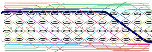
Fig. 3: Non constant crimp of a 9-float Angle Interlock (9A)
