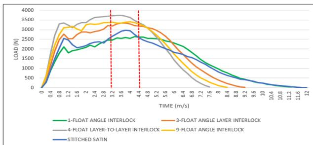
Fig 13: Peak force needed by ogival impactor to penetrate all samples
