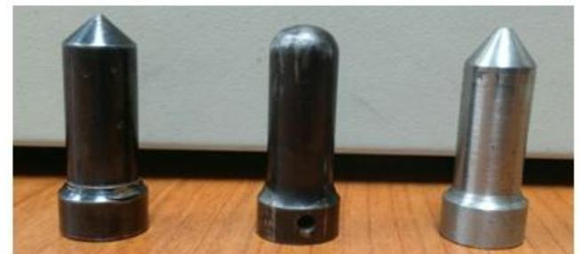
Fig. 6: Ogival (A), Hemispherical (B), Conical (C) Conical impactors
