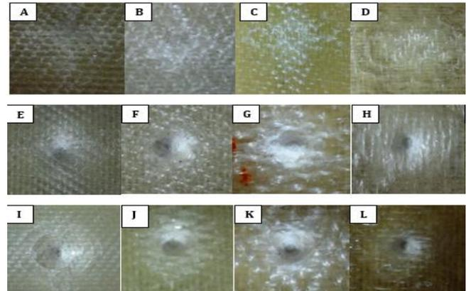
Fig 14: Front Surface Damage on Composites; (A) hemispherical 1A, (B) hemispherical 3AL, (C) hemispherical 4L, (D) hemispherical 9A, (E) conical 1A, (F) conical 3AL, (G) conical 4L, (H) conical 9A, (I) ogival 1A, (J) ogival 3AL, (K) ogival 4L, (L) ogival 9A
