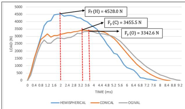
Fig. 8: Peak force over time for all impactor shapes impacted on 3AL composite
