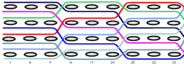
Fig. 2: Non constant crimp of 3-float Angle Layer Interlock (3AL)
