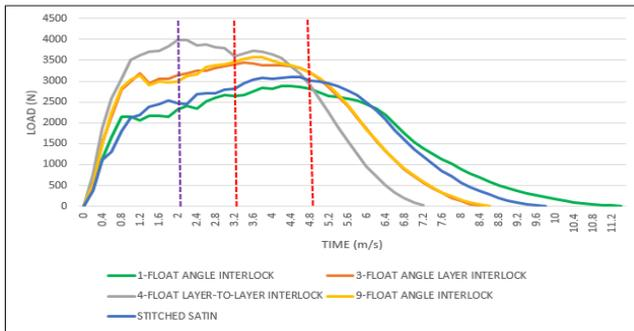
Fig 12: Peak force needed by conical impactor to penetrate all samples
