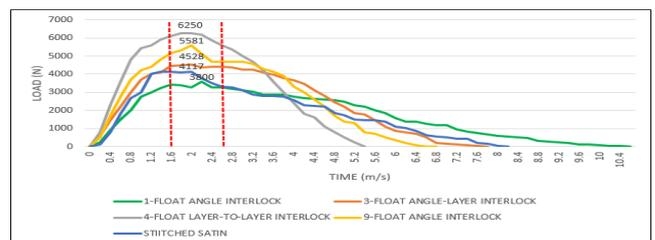
Fig 11: Peak force needed by hemispherical impactor to penetrate all samples
