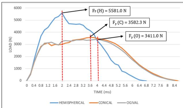
Fig. 10: Peak force over time for all impactor shapes impacted on 9A composite
