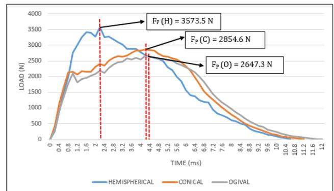
Fig. 7: Peak force over time for all impactor shapes impacted on 1A composite
