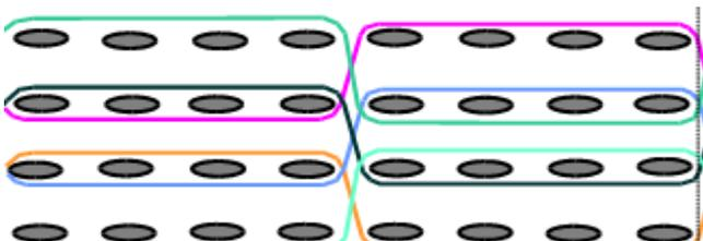
Fig. 4: Non constant crimp of a 4-float Layer-to-Layer Interlock (4L)
