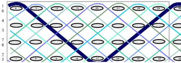
Fig. 1: Non constant crimp 1-float Angle Interlock (1A)
