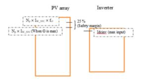
Fig. 5: Matching of PV array current to inverter current.
