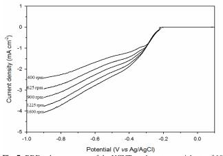
Fig. 7: RDE voltammograms of the NCNT catalyst at potential rate of 10 mV/s and various electrode rotating rates
