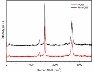
Fig. 3: Raman spectra of CNT and NCNT
