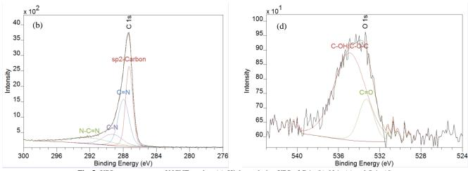
Fig. 5: XPS survey spectra of NCNT catalyst (a), High-resolution XPS of C 1s (b), N 1s (c) and O 1s (d)
