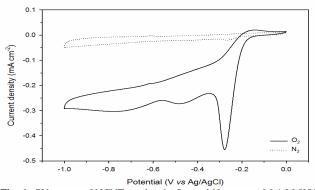
Fig. 6: CV curves of NCNT catalyst in  $O_{2^{\text{-}}}$  and  $N_{2^{\text{-}}}$  saturated 0.1 M KOH aqueous solution at scan rate of 10 mV  $s^{\text{-1}}$
