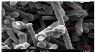
Fig. 2: SEM image of NCNT catalyst
