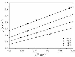
Fig. 8: Koutecky-Levich (K-L) plots of the NCNT catalyst
