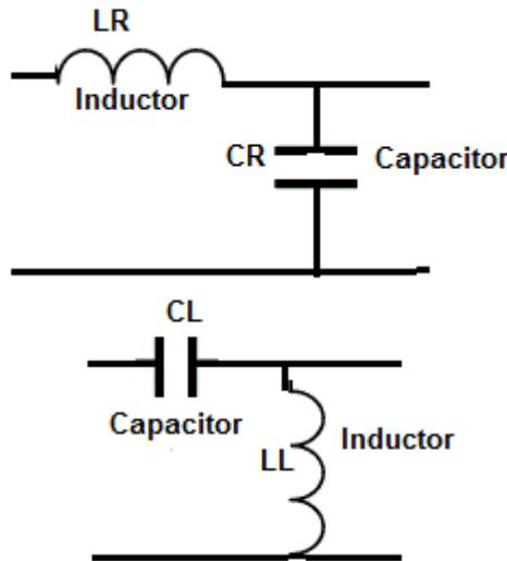
Fig. 2. Equivalent circuits model of a unit cell of (a) RH-TL (b) and LH-TL.
