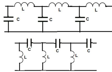
(a) Pure RH transmission line (b) Pure LH transmission line
