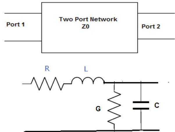
**Figure 7:** (a) Transmission line model: a two-port network, (b) Infinitesimal circuit model of a transmission line
