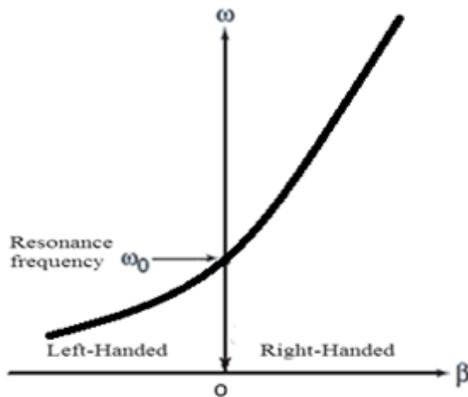
Fig. 4: Typical dispersion diagram of seamless LH to RH transition [23].
