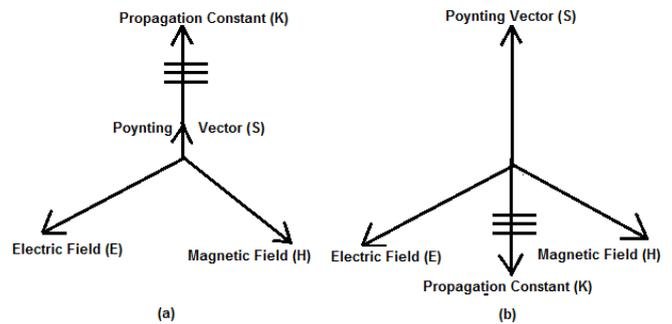
Fig. 3: relation between Electric field (E), magnetic field (H), propagation constant (k), and Poynting vector (S) for (a) Right-handed medium. (b) Left-handed medium
