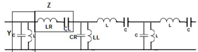
Fig. 6: Equivalent circuit model of composite right/left-handed transmission line
