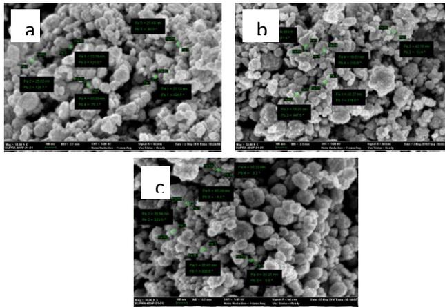
**Fig. 2:** FESEM images of ZnONPs synthesized at temperatures of a) 60°C b) 70°C and c) 80°C
