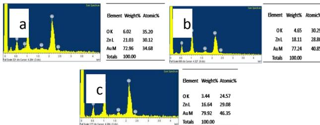
**Fig. 3:** EDX of ZnONPs synthesized at temperature of a) 60°C, b) 70°C and c) 80°C
