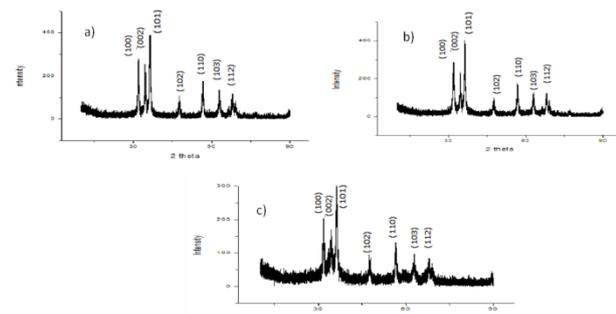
**Fig. 4:** XRD pattern of ZnONPs synthesized at a) 60°C, b) 70°C and c) 80°C.
