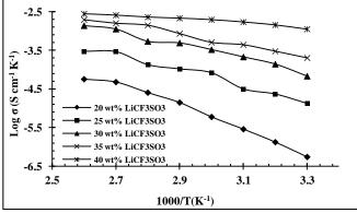
Fig. 2: Arrhenius plot for unplasticized GPE system.
