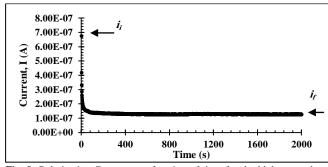
Fig. 8: Polarization Current as a function of time for the highest conductivity of EMG30-LiCF<sub>3</sub>SO<sub>3</sub>.
