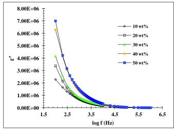
**Fig. 7:** Frequency dependence of dielectric constant at room temperature for 62.3 mol% of EMG30-LiCF<sub>3</sub>SO<sub>3</sub>-x wt.% EC.
