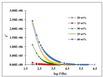
Fig. 6: Frequency dependence of dielectric constant at room temperature for 62.3 mol% of EMG30-x wt.% LiCF<sub>3</sub>SO<sub>3</sub>.
