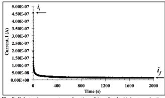
**Fig. 9:** Polarization current as a function of time for the highest conductivity of EMG30-LiCF<sub>3</sub>SO<sub>3</sub>-EC.
