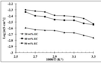
Fig. 3: Arrhenius plot plasticized GPE system.
