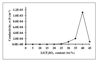
Fig.1: The conductivity plot of the unplasticized EMG30-LiCF<sub>3</sub>SO<sub>3</sub> system.
