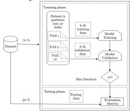
Fig. 5: Process flow diagram for computational experiment. This diagram shows detail process of the modelling SVM
