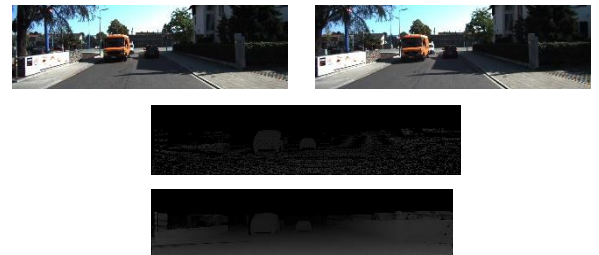
Fig. 7: Up: The left camera image, The right camera image The LIDAR (ground Truth) Predicted Disparity map by the proposed method
