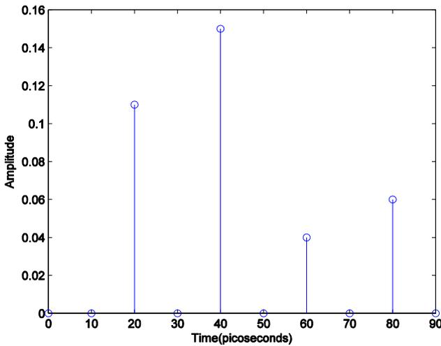
Fig. 4: Multipath channel with sampling rate at 20 picoseconds.
