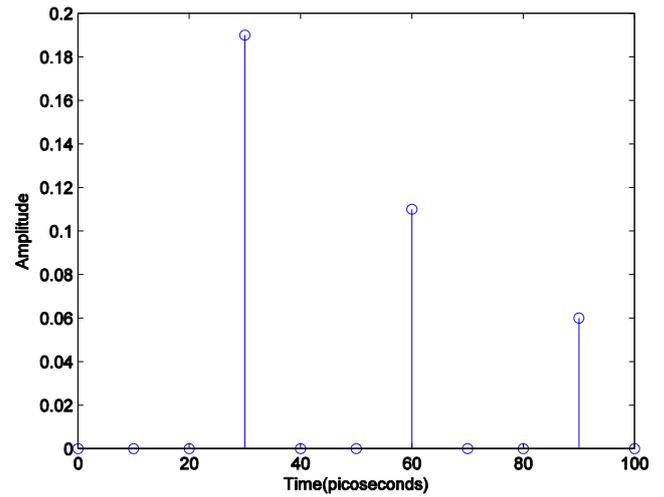
Fig. 4: Multipath channel with sampling rate at 30 picoseconds.
