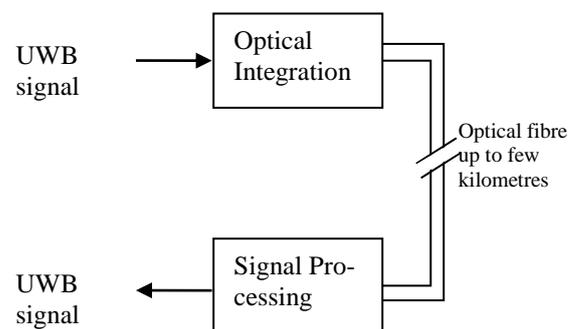
Fig. 1: Integration of UWB signal into optical fibre.
