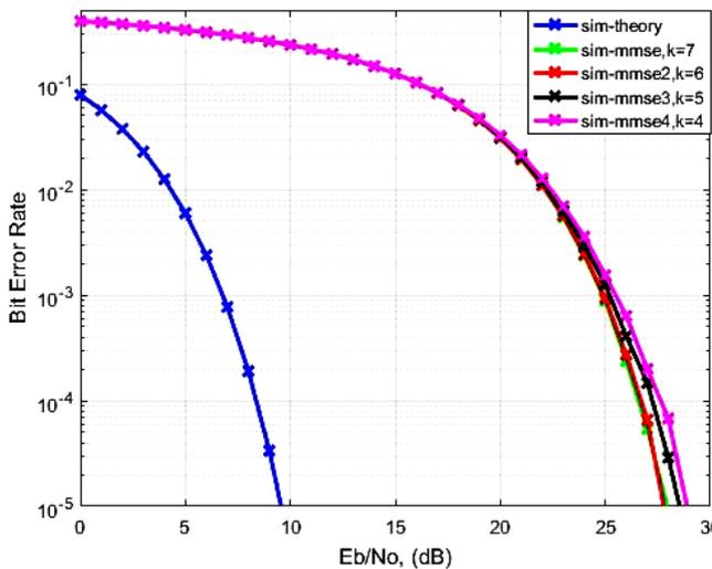
Fig. 5: BER vs  $E_b/N_0$  graph with tap length,  $k = 4, 5, 6$  and  $7$  for second multipath channel.
