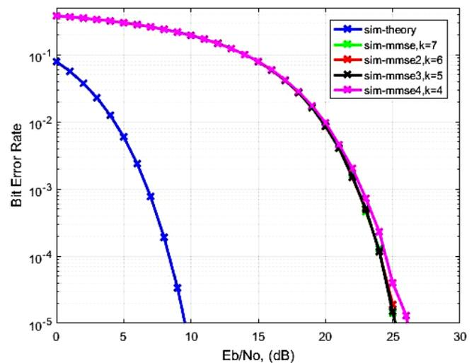
Fig. 5: BER vs  $E_b/N_0$  graph with tap length,  $k = 4, 5, 6$  and  $7$  for third multipath channel.
