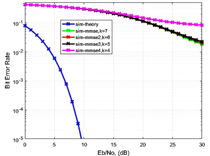
Fig. 3: BER vs  $E_b/N_0$  graph with tap length,  $k = 4, 5, 6$  and  $7$  for first multipath channel.
