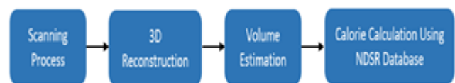
Figure 1. The overall flowchart of the DietSkán system from the scanning process to measuring calorie intake.
