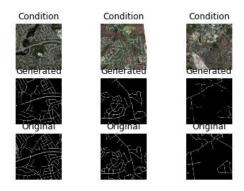
Fig. 7.3: Three aerial images, their generated output from the model, and their corresponding manual vector map outline for epoch 6000
