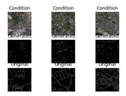
Fig. 7.2: Three aerial images, their generated output from the model, and their corresponding manual vector map outline for epoch 3000
