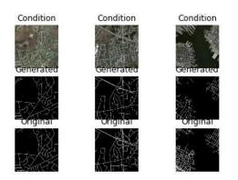
Figure 7.7: Three aerial images, their generated output from the model, and their corresponding manual vector map outline for epoch 24999
