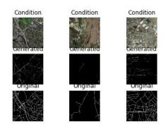
Fig. 7.4: Three aerial images, their generated output from the model, and their corresponding manual vector map outline for epoch 9000
