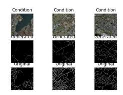
Figure 7.6: Three aerial images, their generated output from the model, and their corresponding manual vector map outline for epoch 18000
