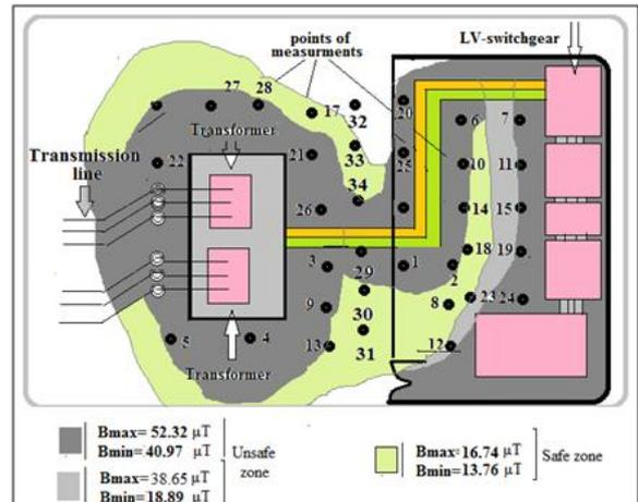
Fig. 5: The safe and unsafe ranges of the electric and magnetic fields emitted from the circuit breaker inside the 132/33 substation
