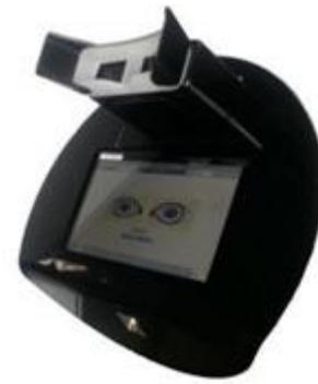
All the three biometrics i.e. face, iris and fingerprint are sometimes scanned by single device otherwise maximum devices can scan face and finger at the same time and for iris scan different device can be used. The hardware components of the device includes platen referred to as scanner which is used to scan fingerprint. CCTV camera required to capture the image of face. Iris scan deployments require special devices that provide necessary infrared illumination.
